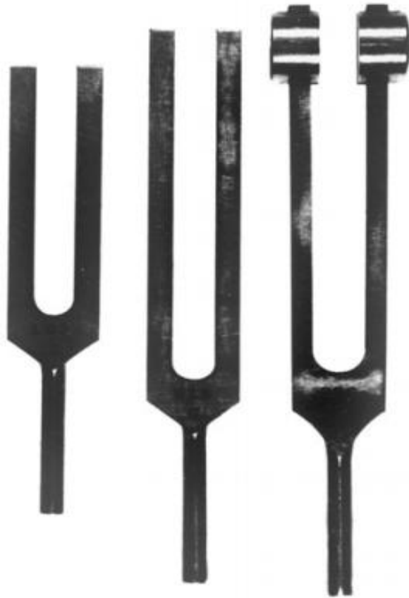
FIGURE 2.3 Several tuning forks. The larger forks vibrate at lower frequencies (produce lower-pitched tones) than the smaller forks.
